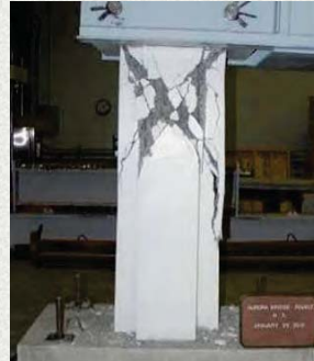
Figure 4. As-Built Column Shear Failure.
