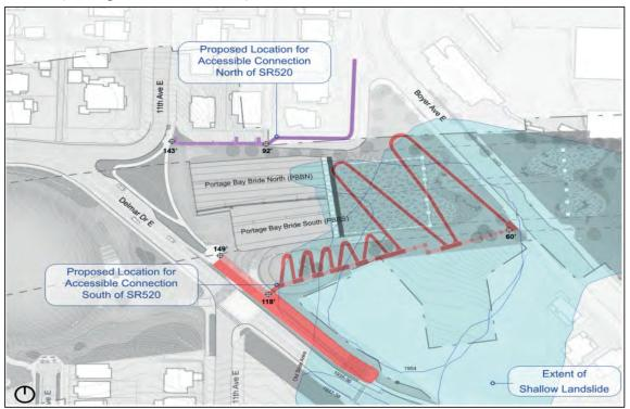
Figure 1. Plan View of Proposed Locations for Boyer/Delmar Accessible Connection (incl. Delmar Landslide Limits)
