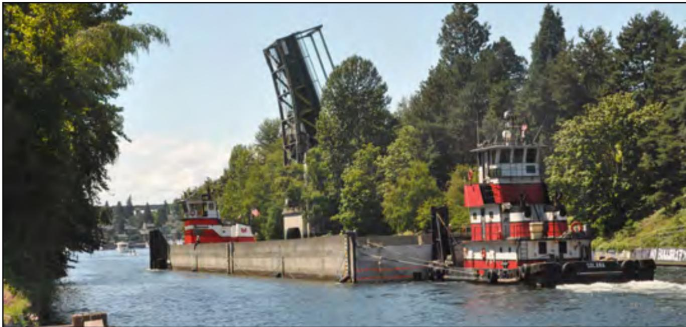
Old floating bridge pontoon E floats through the Montlake Cut on the way to the Hiram M. Chittenden Locks. Photo taken: July 20
