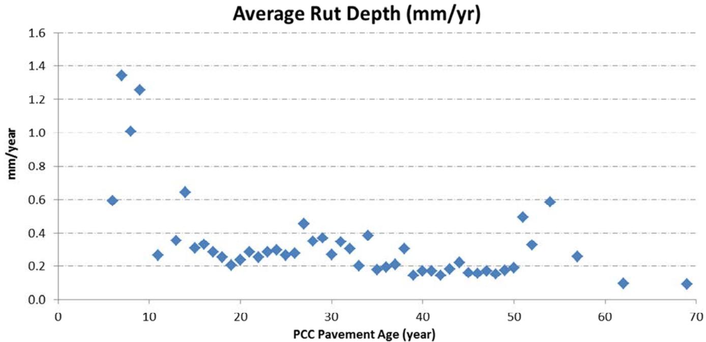
**Figure 1: Plot of average rut depth increase per year (vertical scale, in mm/year) to time (horizontal scale, in years) for concrete pavements.**
