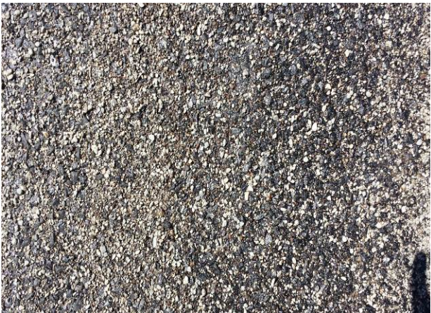
Figure 92. Close-up of choke stone. (August 2016)
