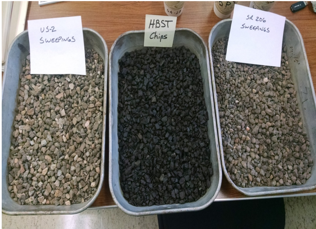
Figure 61. Aggregate sweepings from US-2 (left tray), HBST pre-coated chips (center tray) aggregate sweepings from SR-206 (right tray). (Sept. 2015)
