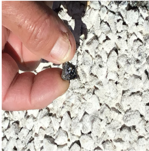
Figure 175. Chip taken from the HBST at MP 7.30 showing 50% embedment. (Aug. 2017)
