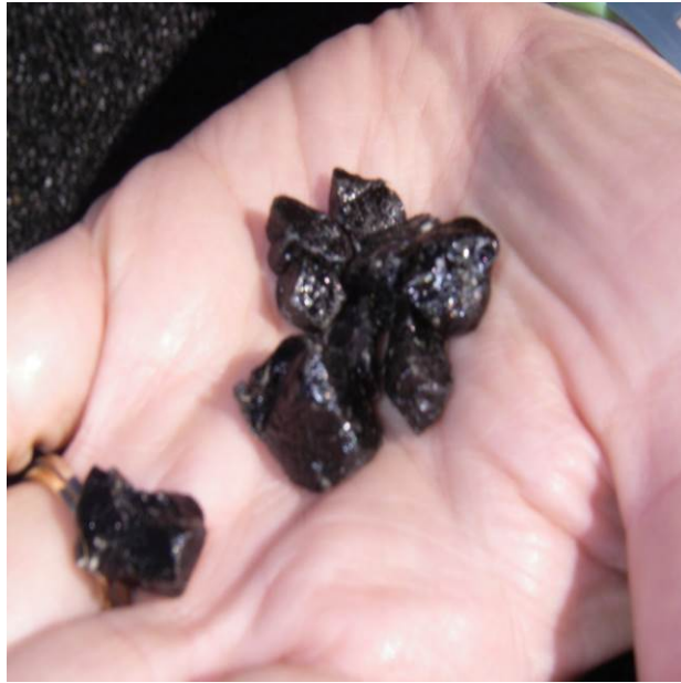
Figure 186. Chips from the shoulder at MP 69.44 with 100% coating. (August 2017)
