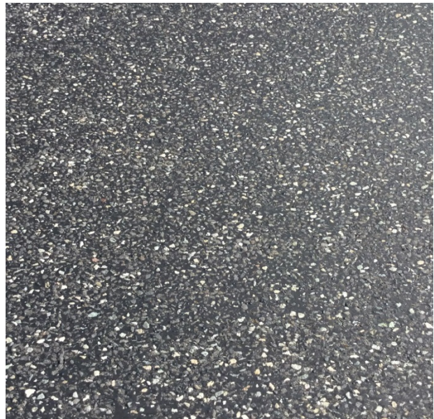
Figure 66. HBST at MP 319.70 with 100% embedment. (August 2017)
