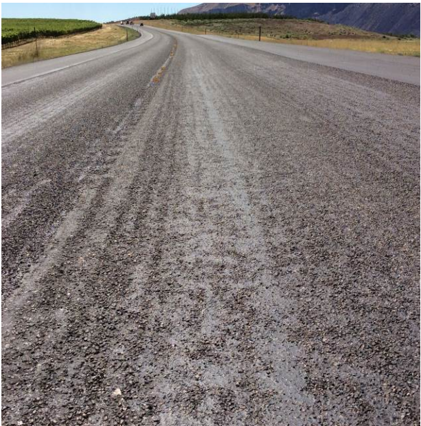
Figure 169. Streaky appearance at MP 18.30. (August 2017)
