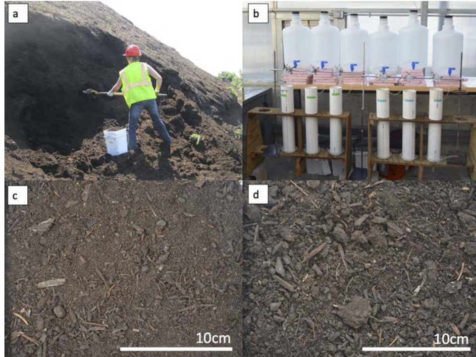
Figure 1: Photos of experiment components. a: compost material collection; b: experimental column setup; c: close-up of 6-month compost; and d: close-up of 24-month compost.
