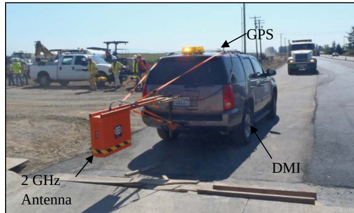
Figure 1 - GPR Equipment Used on this Project
