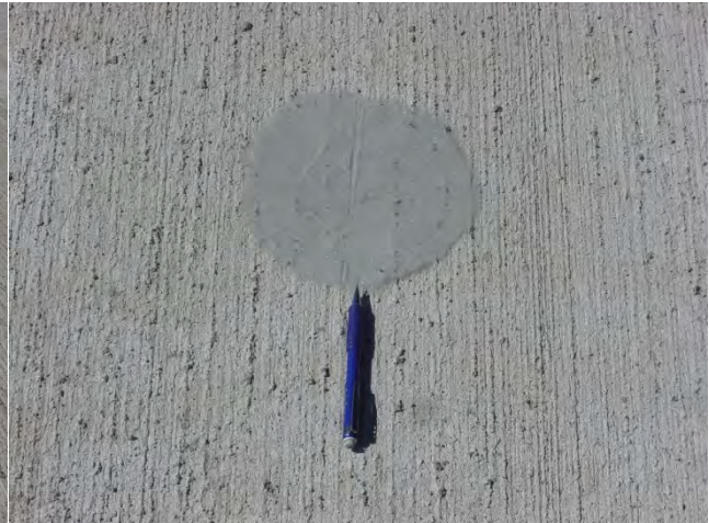
Figure 14. I-5 carpet drag texture close-up of sand patch text.
