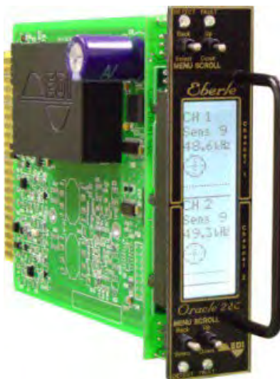
Figure 3-3. EDI Oracle 2E series inductive loop detector
