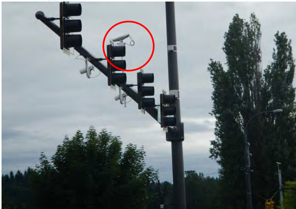
Figure 3-6. Traficon VIP3D.2 sensor
