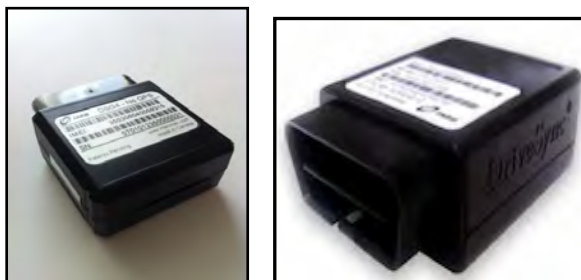
Figure 1: Mileage Reporting Device for Basic (left) and Advanced (right) Road Usage Charge Plan
