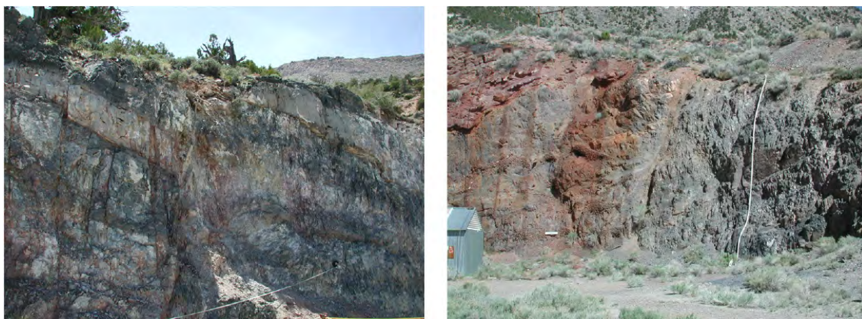
Figure 8.8: Outcrops near U12e tunnel south portal where transects 1 (left) and 2 (right) were used to collect fracture data. Transect 1 is 20 m in length and is orientated approximately N-S; Transect 2 is 15 m in length and is oriented approximately E-W. Data along these two transects was collected from fractures with lengths greater than 0.45 m (1.5 ft).
