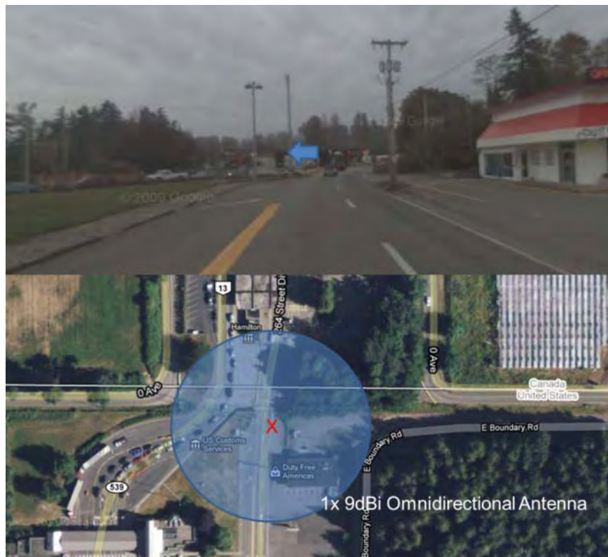
Figure 4-6: SR 539 U.S.-Canada border Bluetooth installation location
