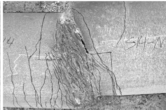
d) Extensive Cracking in Shear Zone
