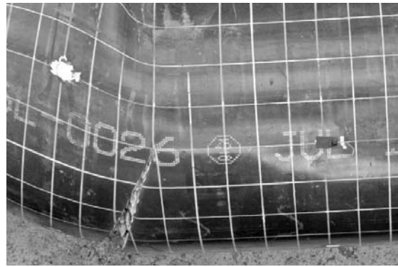
b) Tearing of Steel in Shear Zone
