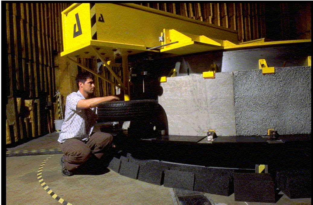
Figure 1. Tire Pavement Test Apparatus (TPTA) located at Purdue University's Herrick Laboratory. (Photo from Purdue University website)
