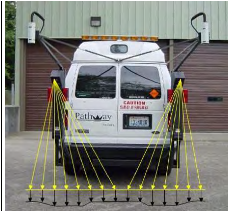
Figure 19. Rut depth measurement using the Pathway Van.
