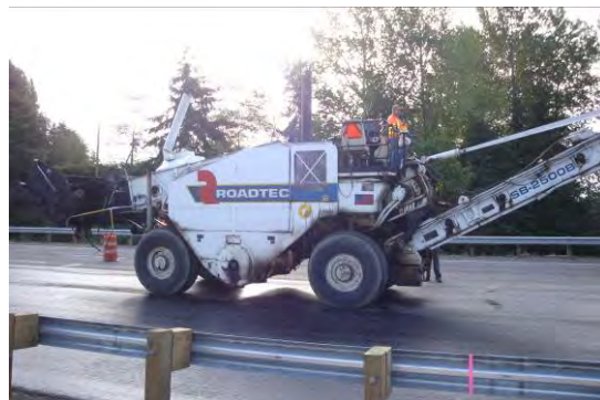
Figure 11. RoadTec Shuttle Buggy.
