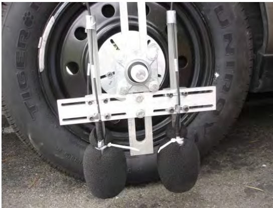
Figure 22. Twin microphones mounted near the rear tire of a vehicle. Note Uniroyal Tiger Paw tire.
