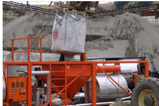
Figure 5. Adding crumb rubber.
