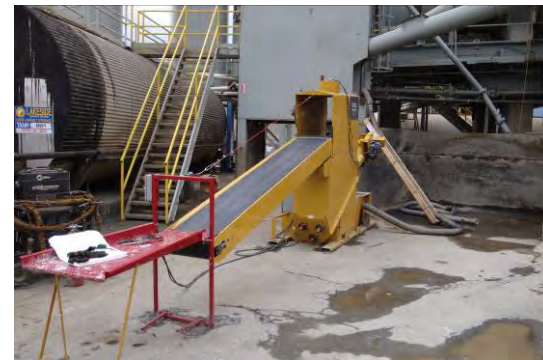
Figure 7. Equipment for introducing fibers into asphalt plant.
