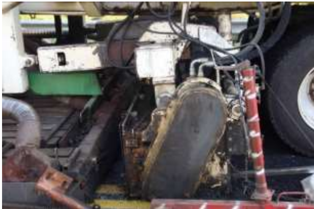
Figure 6. Milling head on left side of unit A.
