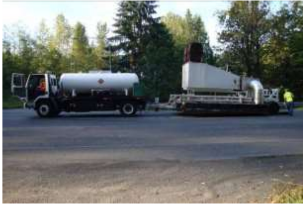
Figure 2. Preheater unit consisting of a propane truck and trailer with propane fired heaters.
