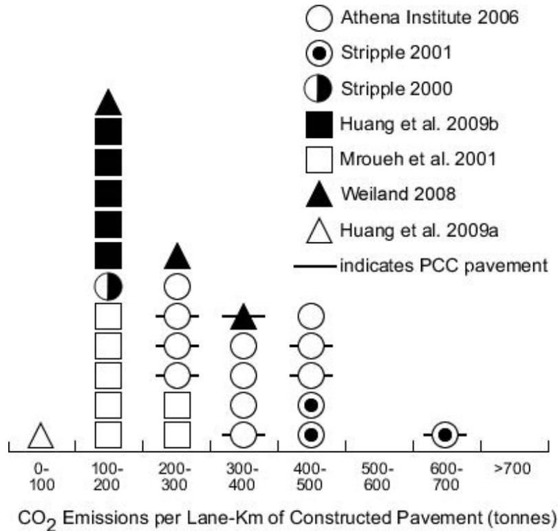
**FIGURE 7. Histogram of CO<sub>2</sub> emissions per lane-km of constructed pavement for 32 assessments in seven pavement LCA papers. Each symbol represents one assessment.**
