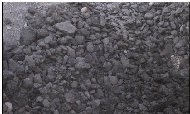
Figure 14. Material that did not pass through the RAP screen.
