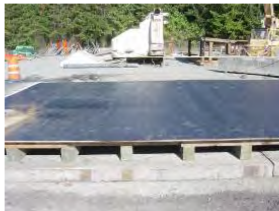
Figure 4. Simulated orthotropic bridge deck.
