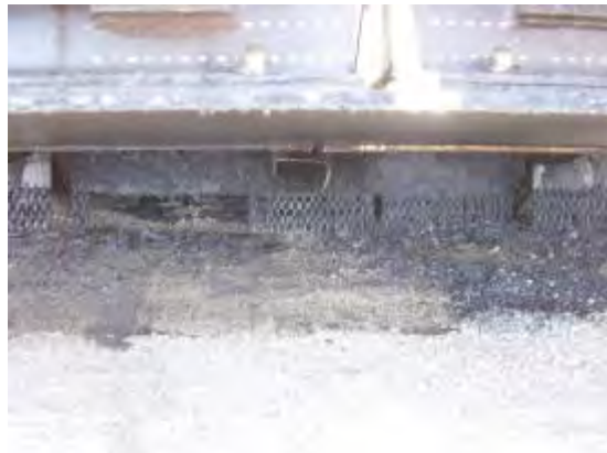
Figure 14. Missing chains on MMK retrofit.
