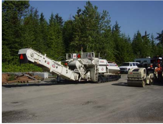
Figure 10. Terex/Cedarapids CR662RM RoadMix transfer vehicle.
