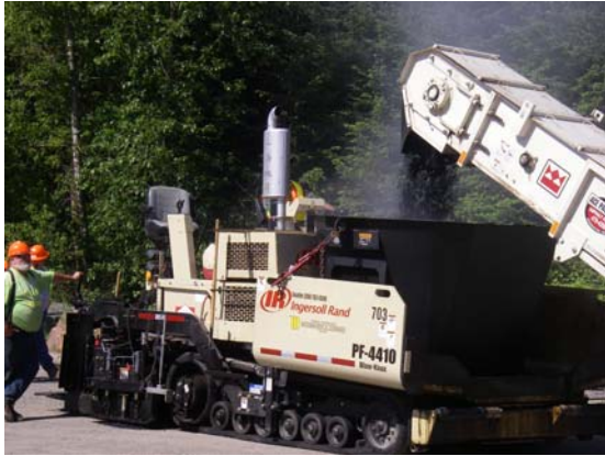
Figure 9. Ingersoll-Rand/Blaw Knox PF-4410 paver.
