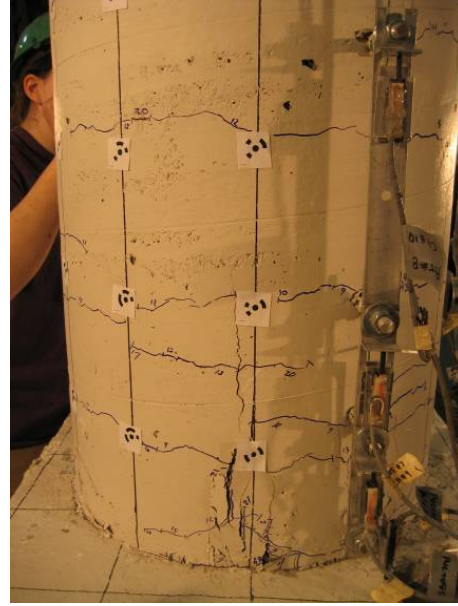
Figure 4-14. LB6-PT: Cycle 24 (4.17%), compression side.
