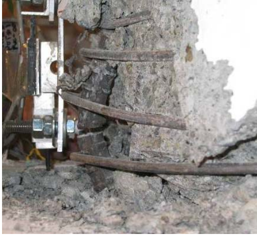
Figure 4-8. LB7-PT: Bar V00 fracture, Cycle 35 ( 2.11%).
