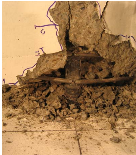
Figure 4-7. LB7-PT: spiral fracture, Cycle 32 (-5.32%).
