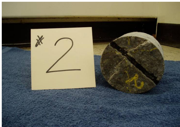
Figure 4. End view showing joint and crack. August 2004
