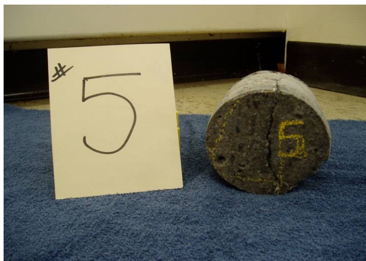
Figure 10. End view showing cracks. August 2004
