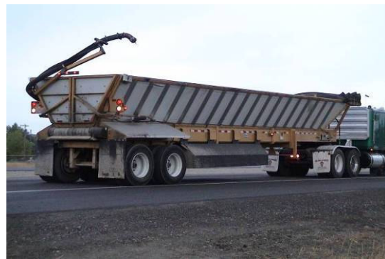
Image D. Aggregate truck with asphalt storage tank below. The hose rotates to connect to the paving machine to transfer the binder.
