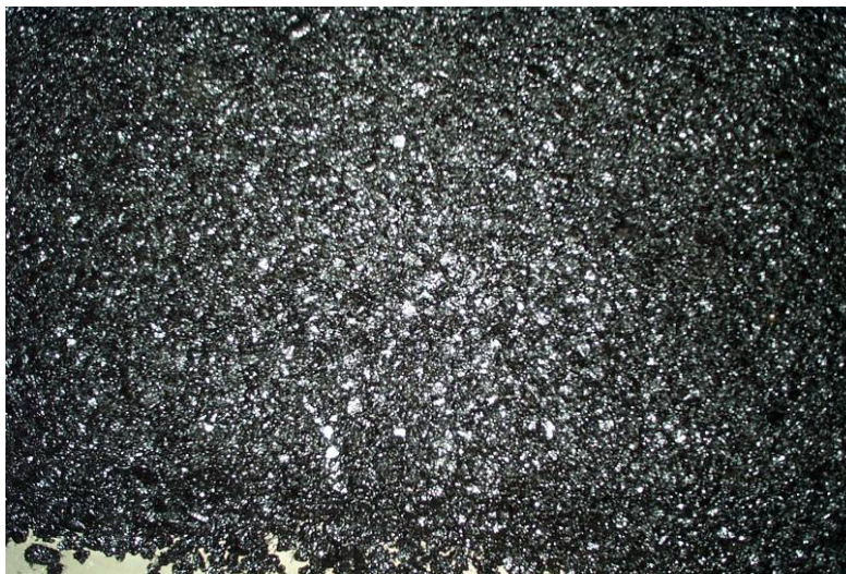
Figure 6. Close-up of Modified Class D mix.
