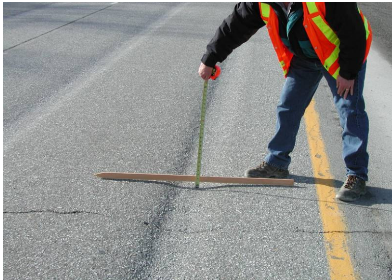
Figure 1. Studded tire wear in HMA pavement on I-90 near the Idaho border.
