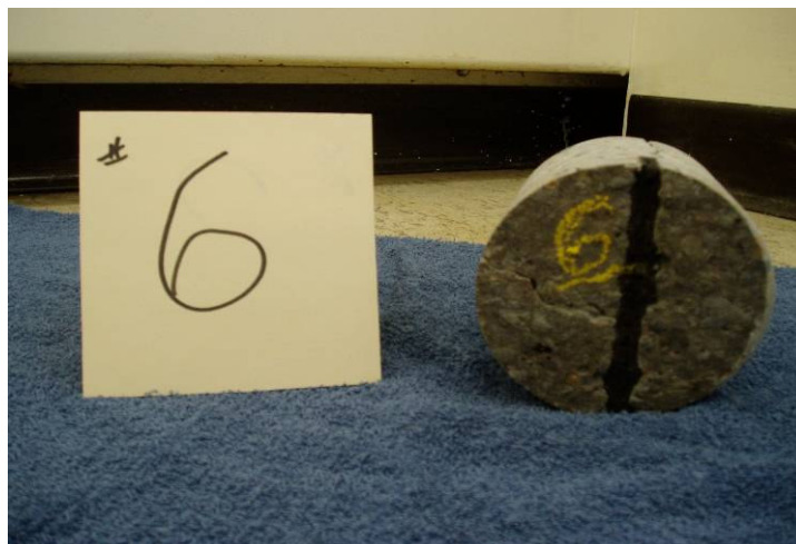
Figure 12. End view showing joint and cracks. 8/04
