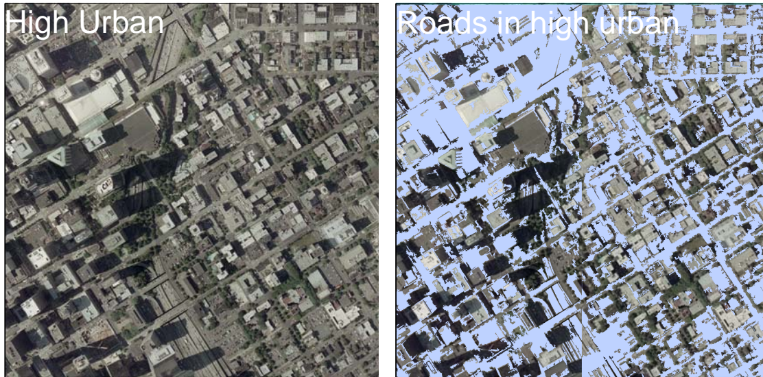
Figure 5. Roads extraction from aerial photo using Feature Analyst ® 4.0 in a urban scene.
