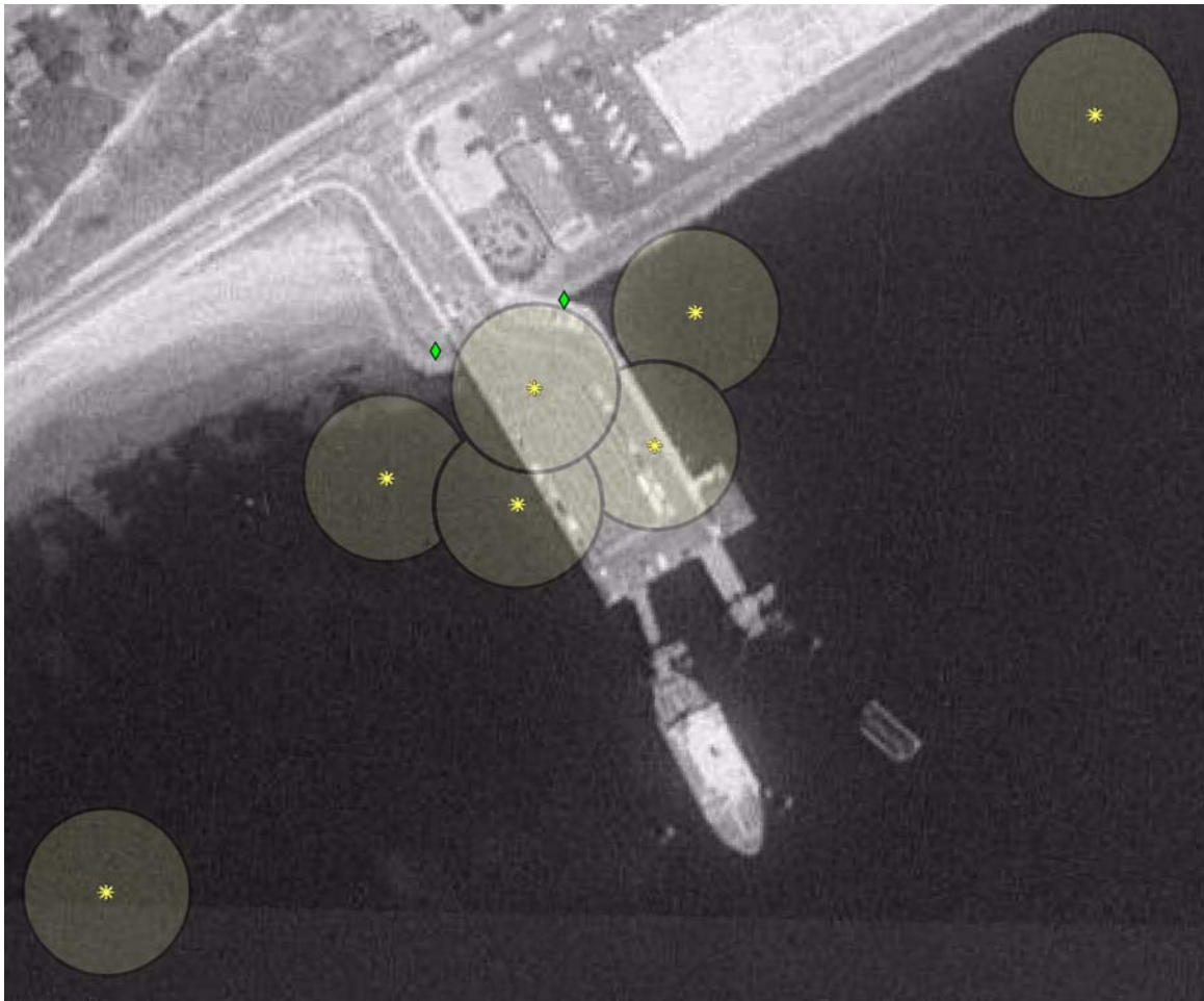
Figure 12. Acoustic Receiver (node) Placement and Estimated Ranges (shaded circles) at the Port Townsend Ferry Terminal.
