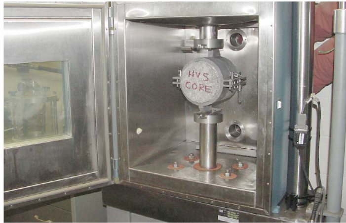
Figure 2.2: FDOT Shear Tester device inside an MTS (Courtesy of FDOT).
