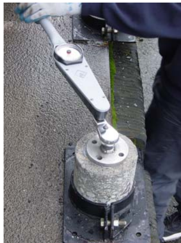
Figure 2.5: WSDOT personnel performing the Torque Bond test.
