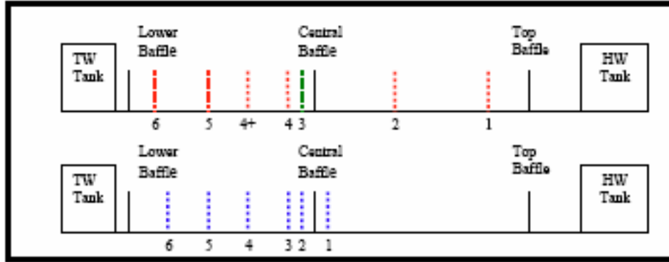
Figure 7. Hydraulic Measurement Locations. Water flows from right to left. Solid lines are baffles; dotted green line = fine grid; dotted red lines = coarse grid; dotted blue lines = super-fine grid.
