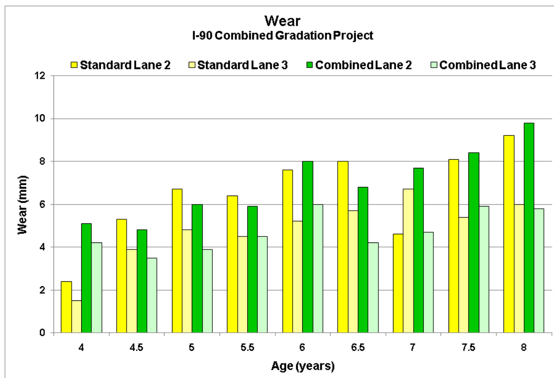
Figure 9. Wear measurements for the I-90 Combined Gradation Project.
