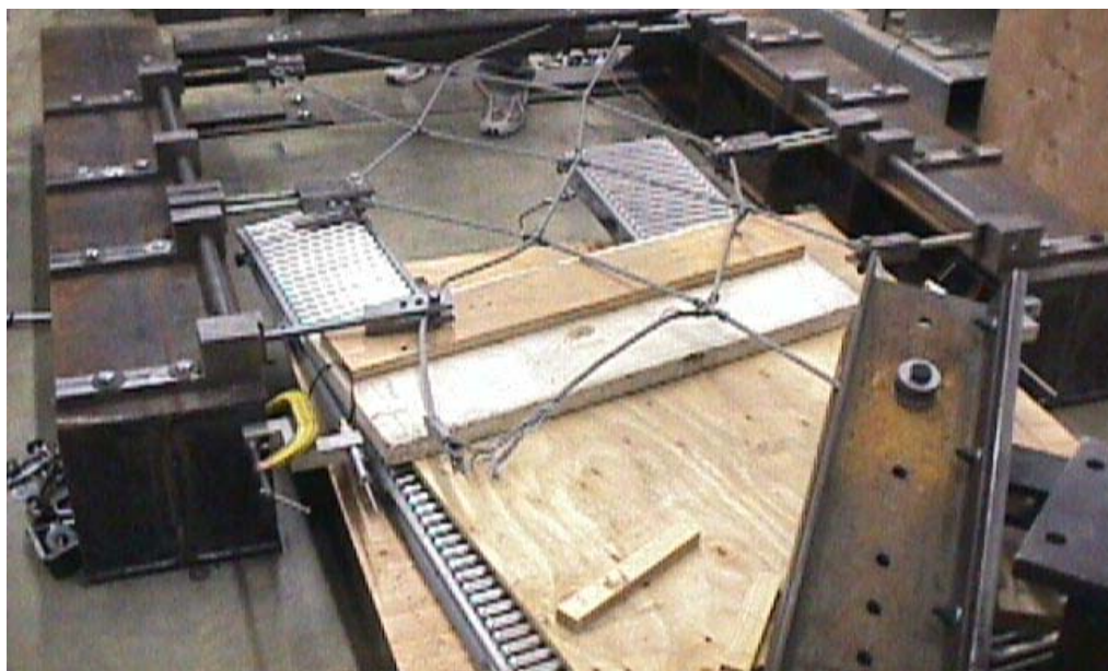
Figure 10. Typical Cable Failure of Maccaferri Cable Net Specimens
