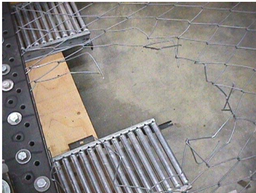
Figure 6. Typical Failure for GeoBrugg Twist Meshes
