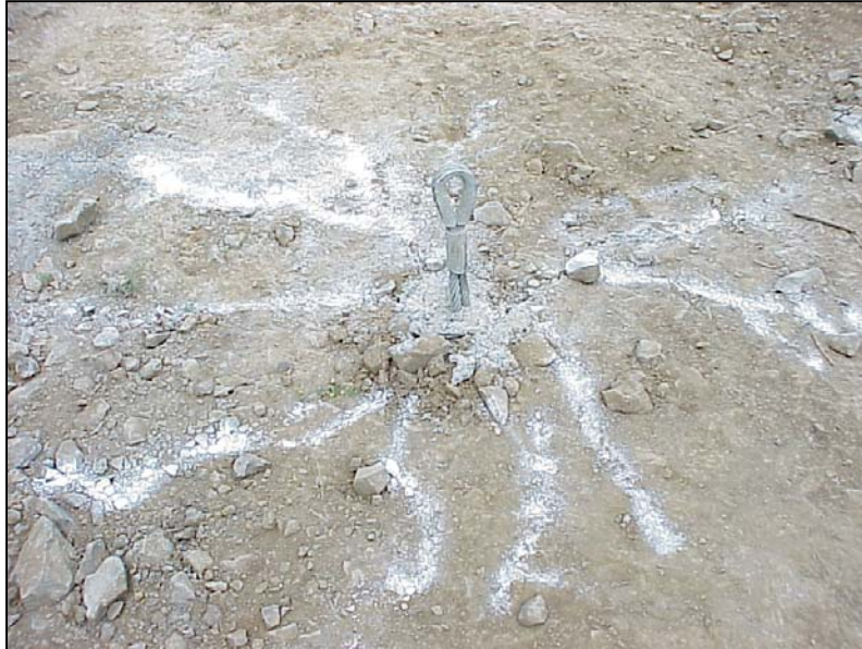
Figure 3-18. Ground cracking (white painted lines) that developed around Anchor 17 (double cable anchor) during vertical loading.
