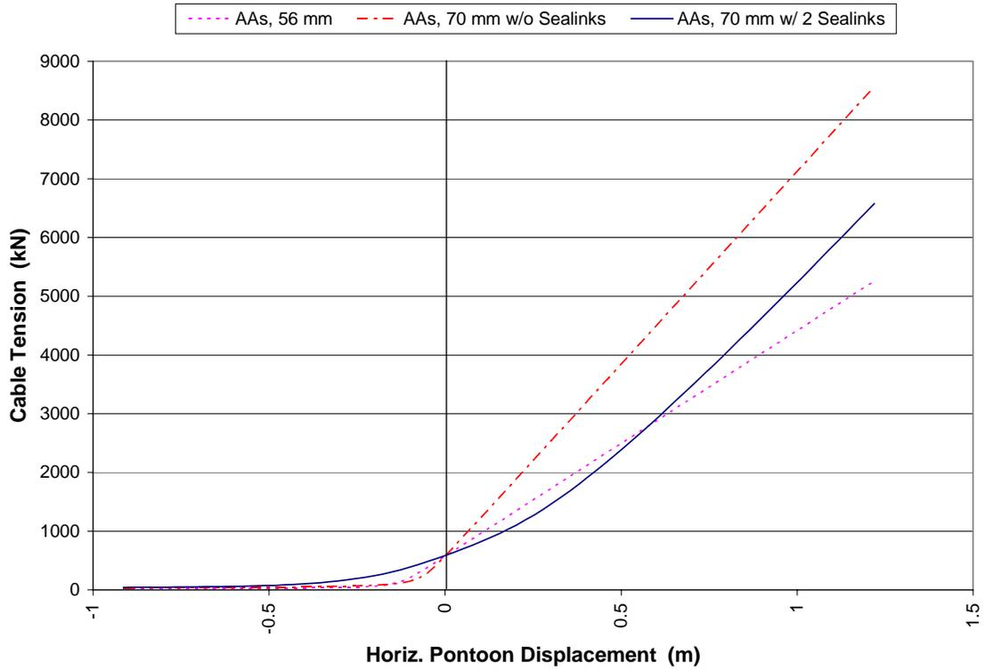
**Figure B.7 – Cable Tension vs. Horizontal Pontoon Displacement, Cable AAs**
