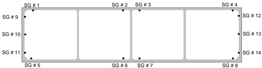
**Figure 5 – Locations of Flexural Strain Gages**
