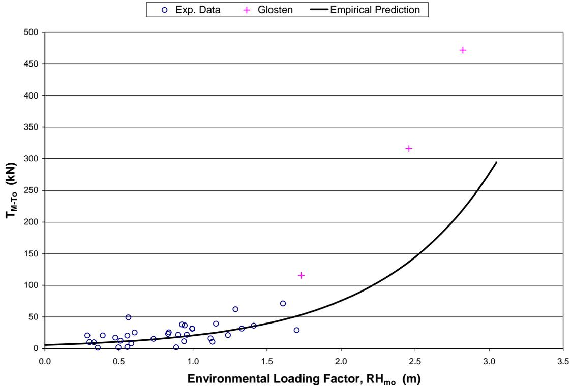
Figure A.7 -  $T_{M-To}$  vs. Environmental Loading Factor, Cable  $R_s$
