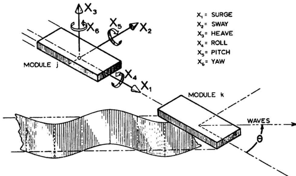
**Figure 3 – Coordinate System and Degrees of Freedom for Structural Model
