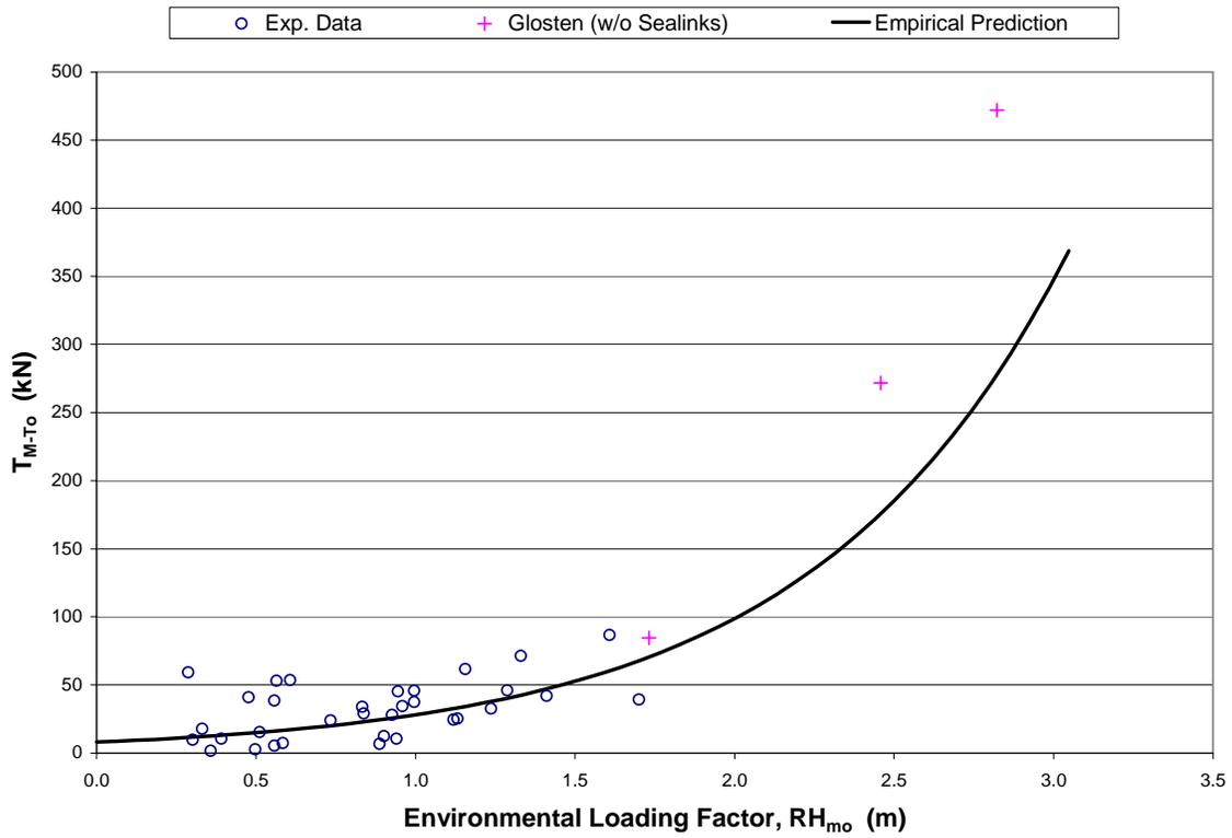
Figure A.13 -  $T_{M-To}$  vs. Environmental Loading Factor, Cable AA<sub>s</sub>
