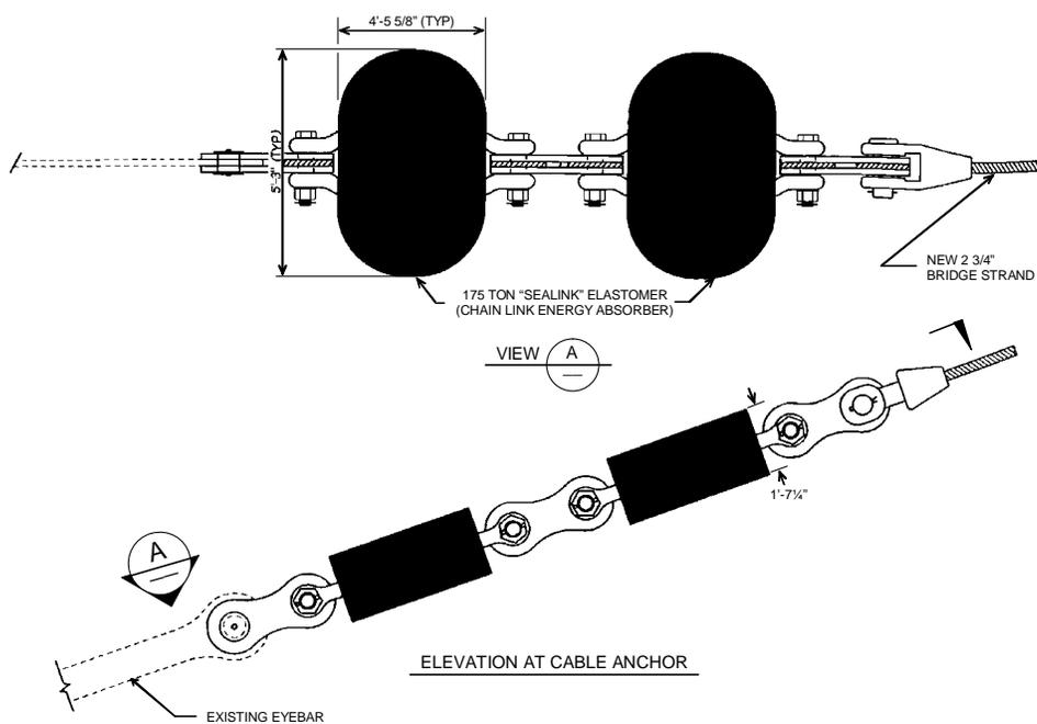
**Figure 2 – Elastomers Installed in Series with Mooring Cable**
