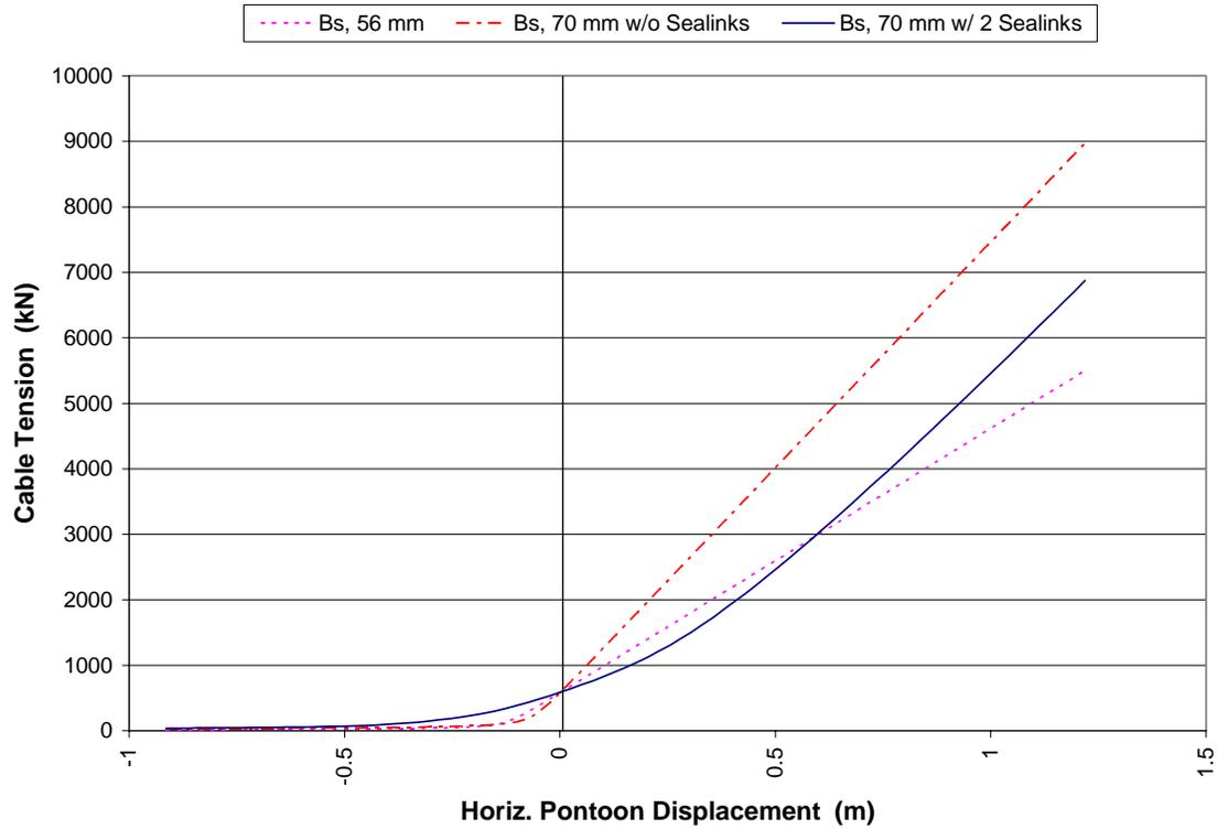
**Figure B.3 – Cable Tension vs. Horizontal Pontoon Displacement, Cable B<sub>s</sub>**
