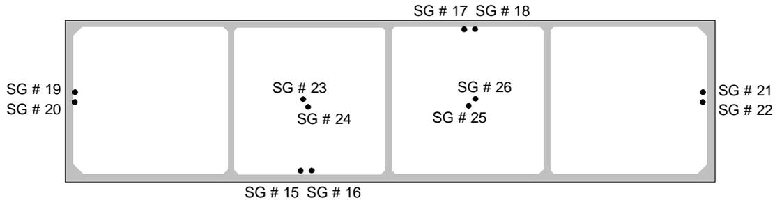
**Figure 6 – Locations of Shear Strain Gages**
