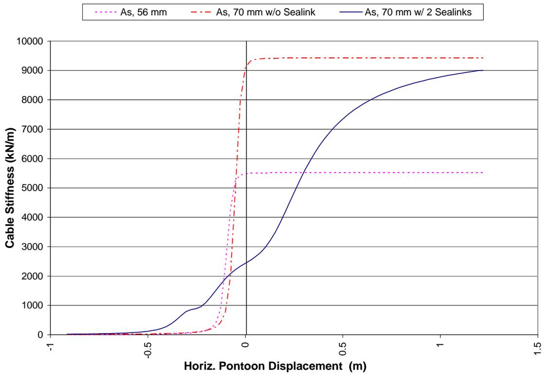
**Figure B.2 – Cable Stiffness vs. Horizontal Pontoon Displacement, Cable A<sub>s</sub>**
