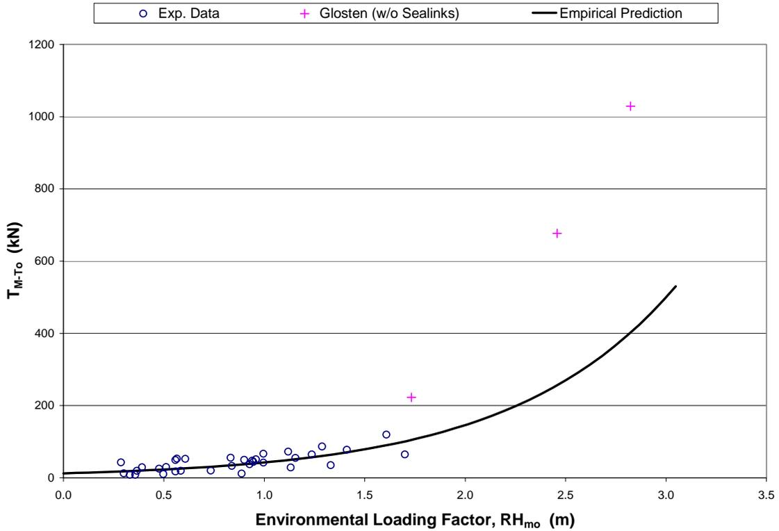
**Figure A.1 -  $T_{M-To}$  vs. Environmental Loading Factor, Cable  $B_s$**
