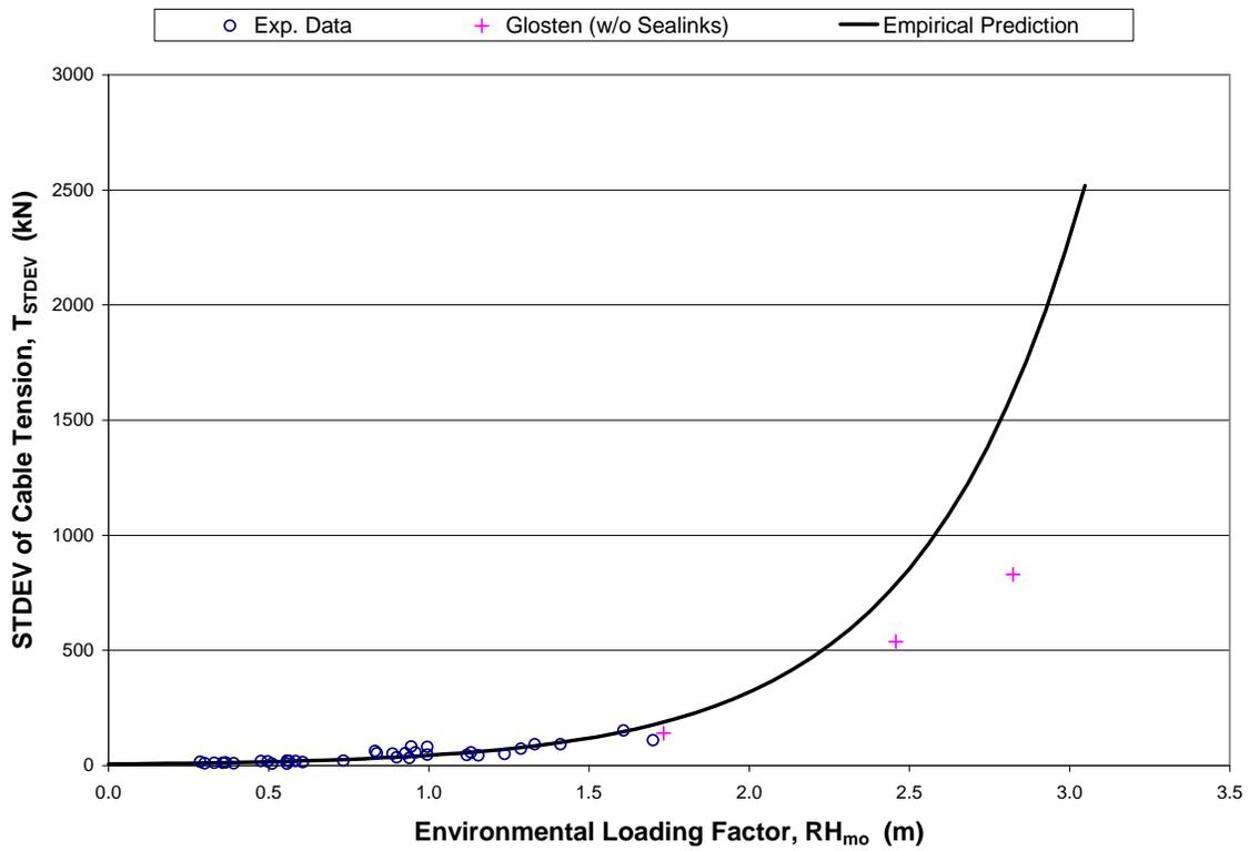
Figure A.14 -  $T_{STDEV}$  vs. Environmental Loading Factor, Cable AA<sub>s</sub>
