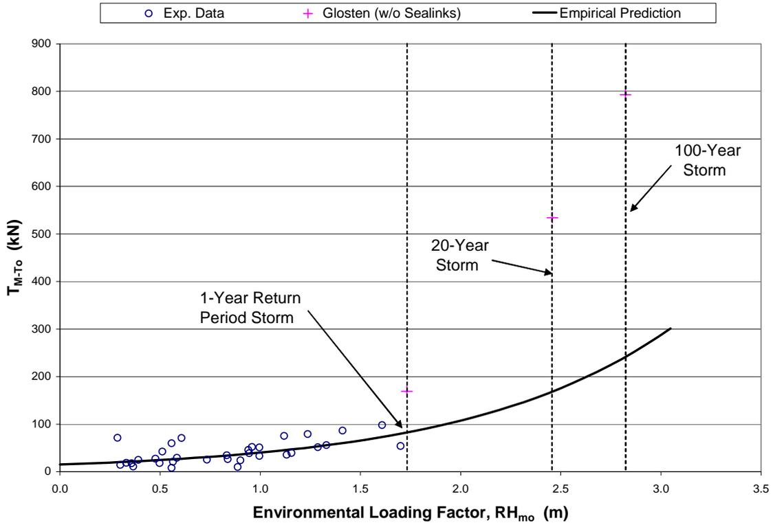
Figure 8 -  $T_{M-To}$  vs. Environmental Loading Factor, Cable  $A_s$
