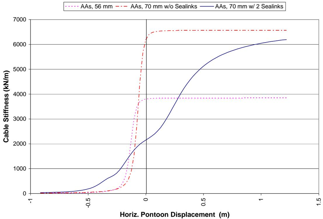
**Figure B.8 – Cable Stiffness vs. Horizontal Pontoon Displacement, Cable AAs**
