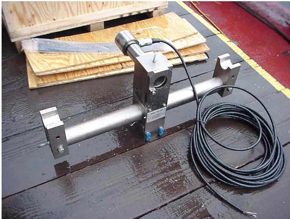
**Figure 4 – Tensiometer Instrument**
