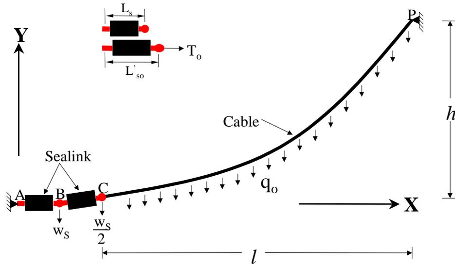
**Figure 10 – Structural Model of Mooring Cable and Sealinks**
