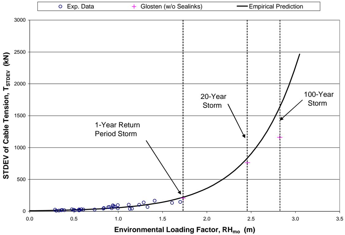
Figure 9 -  $T_{STDEV}$  vs. Environmental Loading Factor, Cable  $A_s$
