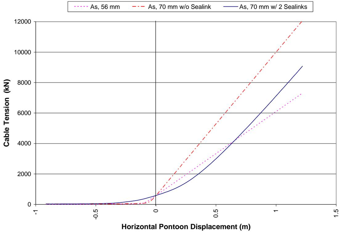
**Figure B.1 – Cable Tension vs. Horizontal Pontoon Displacement, Cable A<sub>s</sub>**
