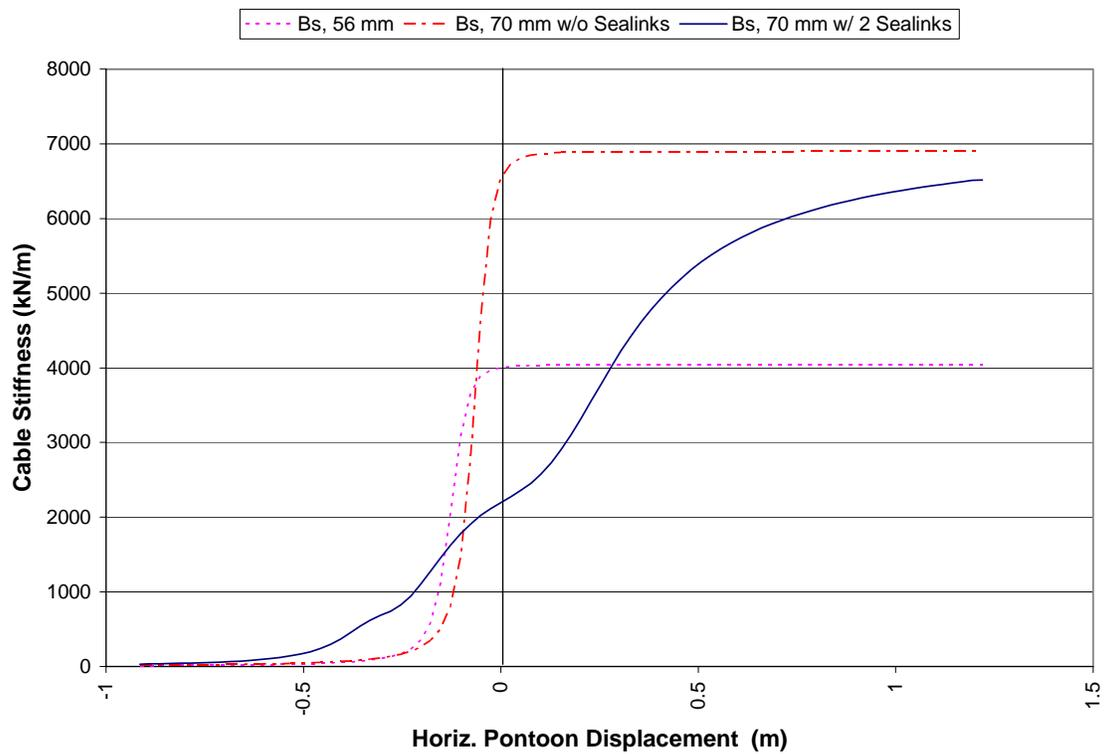
**Figure B.4 – Cable Stiffness vs. Horizontal Pontoon Displacement, Cable B<sub>s</sub>**
