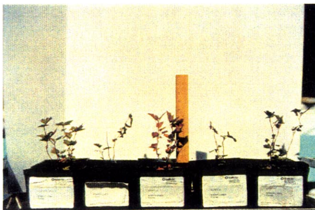
Figure. F.16. Week 11 P. capitatus in potting soil and gasoline-contaminated test soils 9-12 (9 untreated control, 10 mycoremediation, 11 bioremediation, and 12 enhanced bacterial treatment) from left to right
