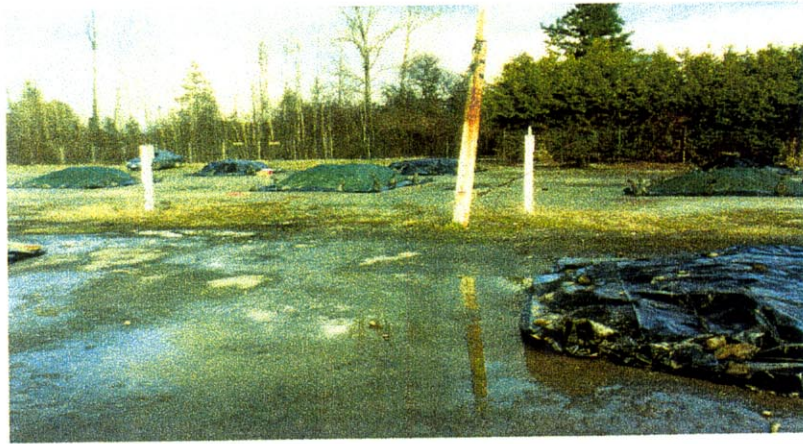
Figure 4. Time 0 bacterial (foreground), mycoremediation (65% green shade cloth), and control (background, with black polyfilm) mounds and their covering
