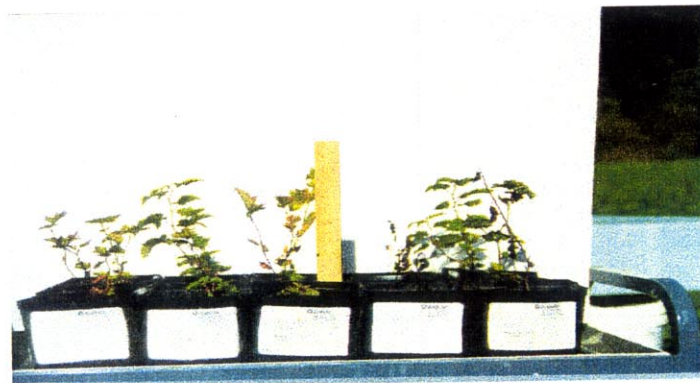
Figure F.14. Week 11 Physocarpus capitatus in potting soil and truck bay test soils (1 untreated control, 2 mycoremediation treatment, 3 bioremediation, and 4 enhanced bacterial treatment) from left to right
