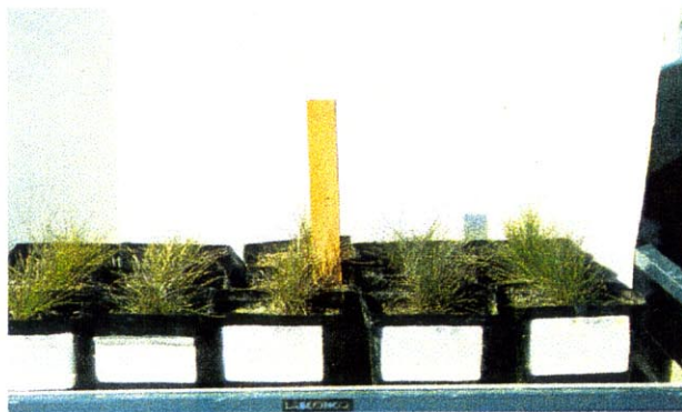
Figure F.8. Week 11 F. idahoensis on potting soil and gasoline-contaminated test soils (9 untreated control, 10 mycoremediation, 11 bioremediation, and 12 enhanced bacteria treatment) from left to right
