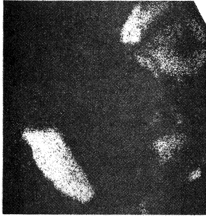
Figure C6. X-Ray Scan for Sulfur (Sample, location and magnification same as Figure C5)
