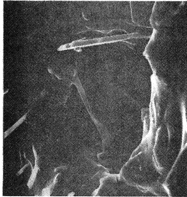
C36. SEA 30/70 Mixture (AR-4000, crushed basalt, Marshall compaction) After Heat Soaking (1,040x).
