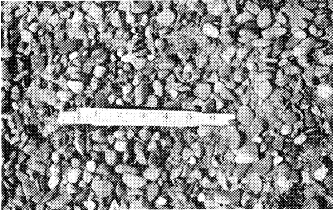
FIGURE 9. THE APPEARANCE OF THE SPECIAL SCREENED NON-FRACTURED AGGREGATE AT THE TEST TRACK STOCKPILE.
