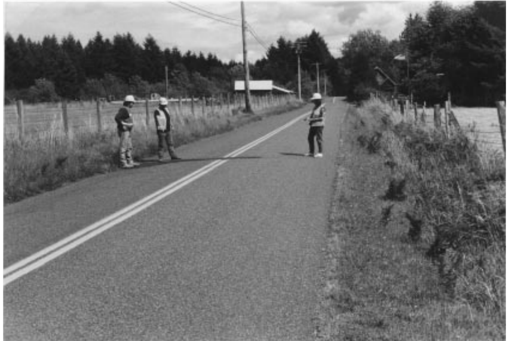
A walking visual inspection of the roadway segment will provide highly accurate pavement condition data.
