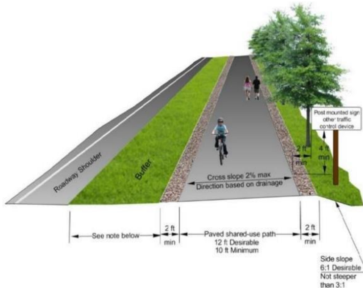
Exhibit 1515-5 Two-Way Shared-Use Path: Adjacent to Roadway (> 35 mph)
