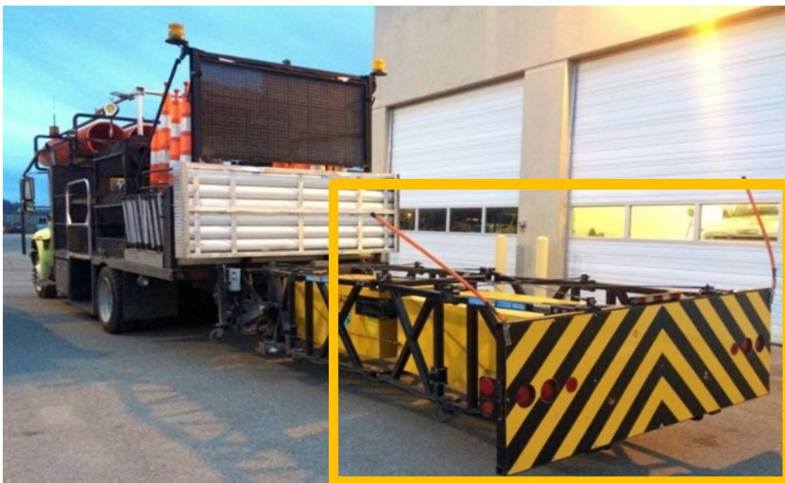
Highlighted Example: TMA attached behind a Traffic Control Placement Vehicle.
