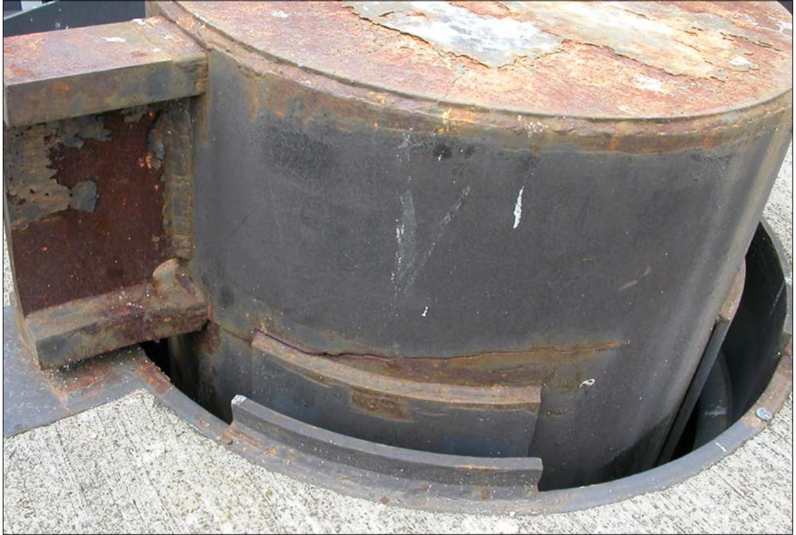
Figure 17 Cracked Reaction Pile
