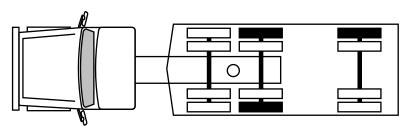
Either drive axle, one tire on each side of the same axle, and one tire on either side of the trailer.
