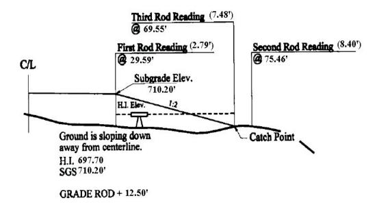
Figure 15-3 Slope stake Example
