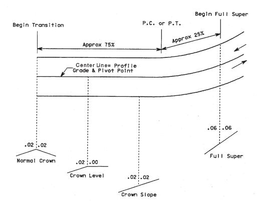
Superelevation for Two-Lane Highway Figure 11-10
