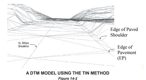
Breaklines define the points where slopes change in grade (the intersection of two planes). Examples of Breaklines are the crown of pavement, edge of pavement, edge of shoulder, flow line, top of curb, back of sidewalk, toe of slope, top of cut, and top of bank. Breaklines within existing highway rights of way are clearly defined, while breaklines on natural ground are more difficult to determine.
