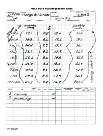
Figure 15-1 Field Notes for Clearing and Grubbing
