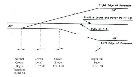
Superelevation Diagram for Two-Lane Highway Figure 11-11
