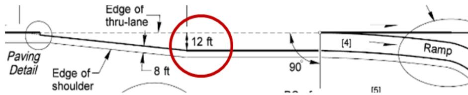
Example: [Exhibit 1360-21](#) calls out one specific dimension for the lane width of this section of a parallel off connection.
