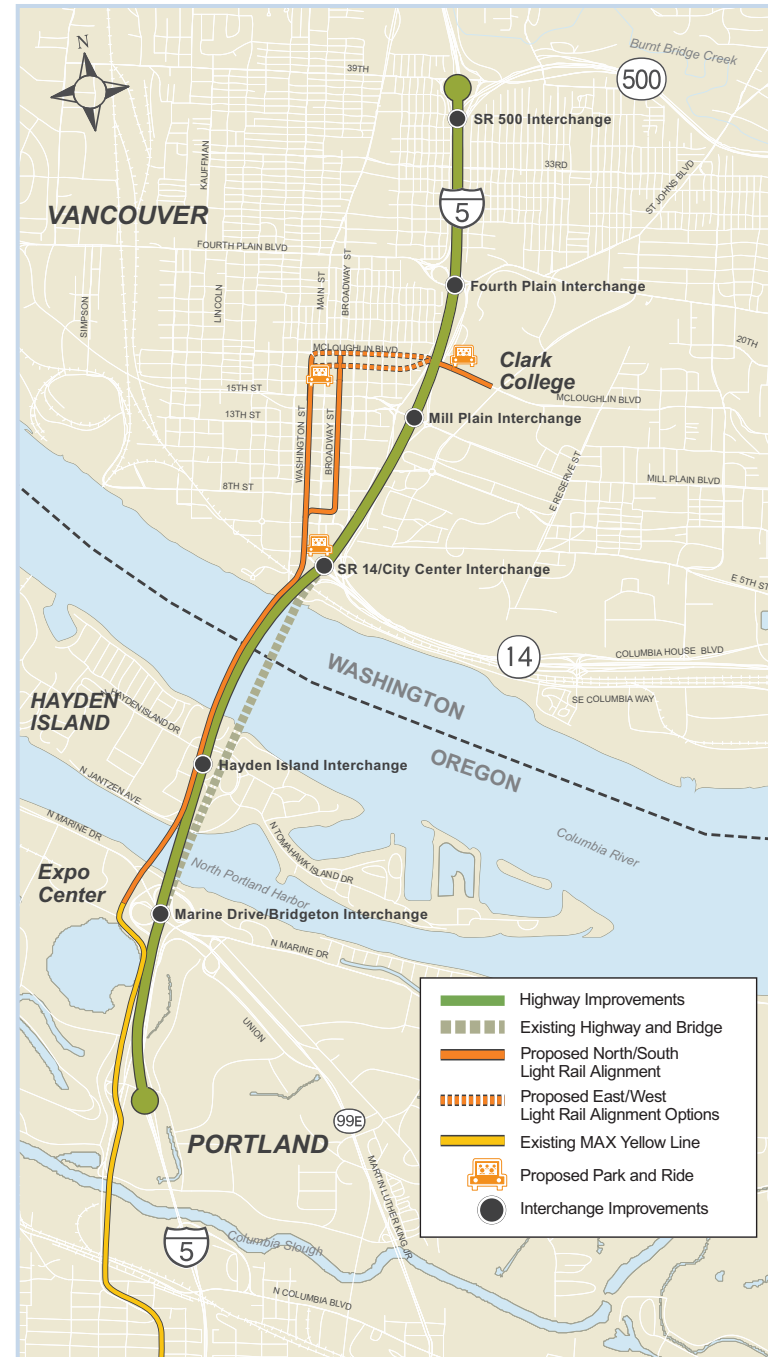
The CRC project area is a five-mile segment of I-5 from Columbia Boulevard in Portland to SR 500 in Vancouver.
