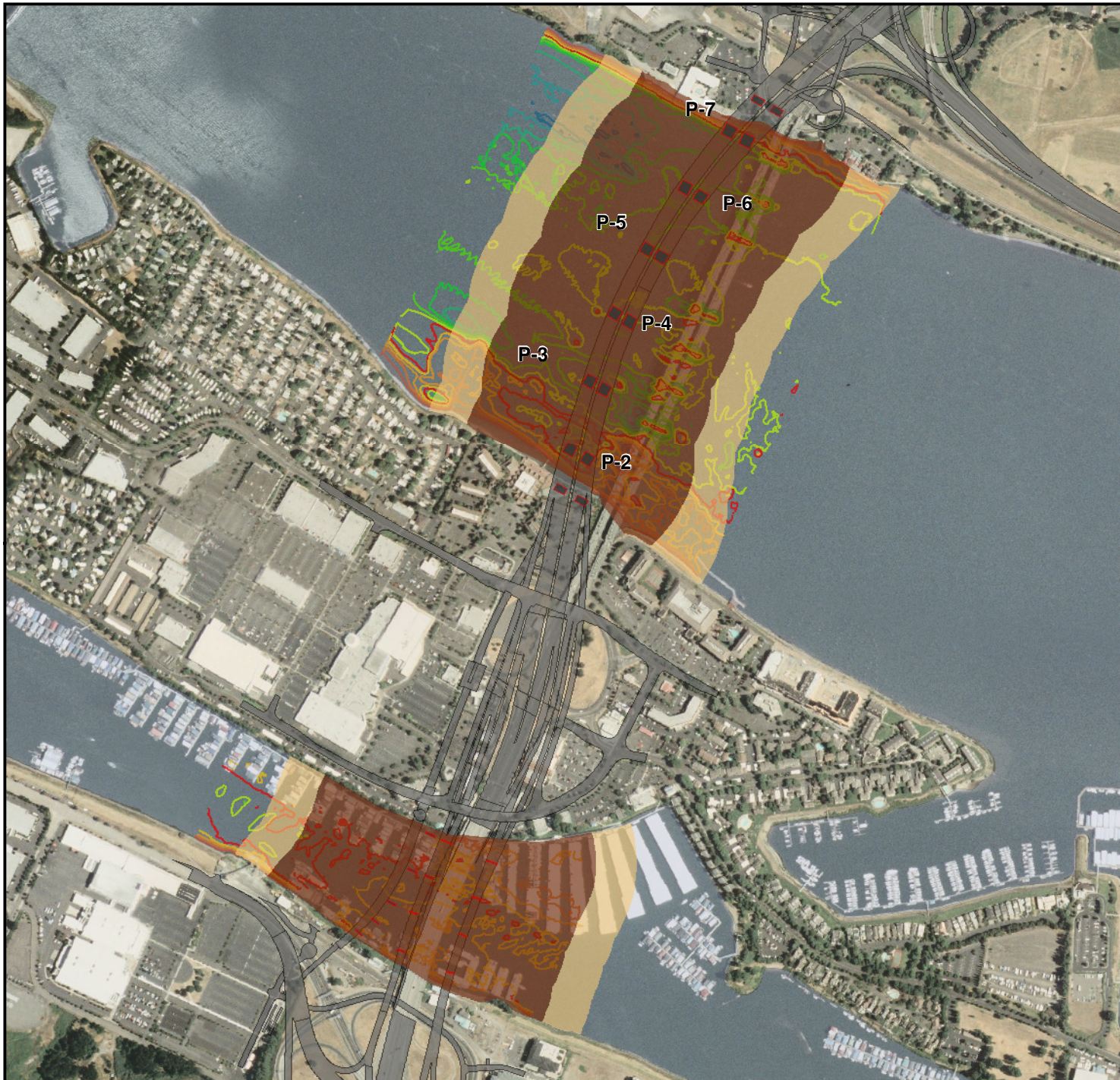
Exhibit 5-45. Extent of airborne impact pile-driving noise exceeding 100 dB RMS disturbance threshold for California and Steller sea lions.
