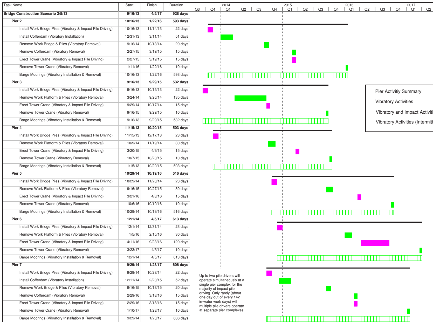
Figure 5-23. Sequencing of Pile Driving and Removal for Construction in the Columbia River
