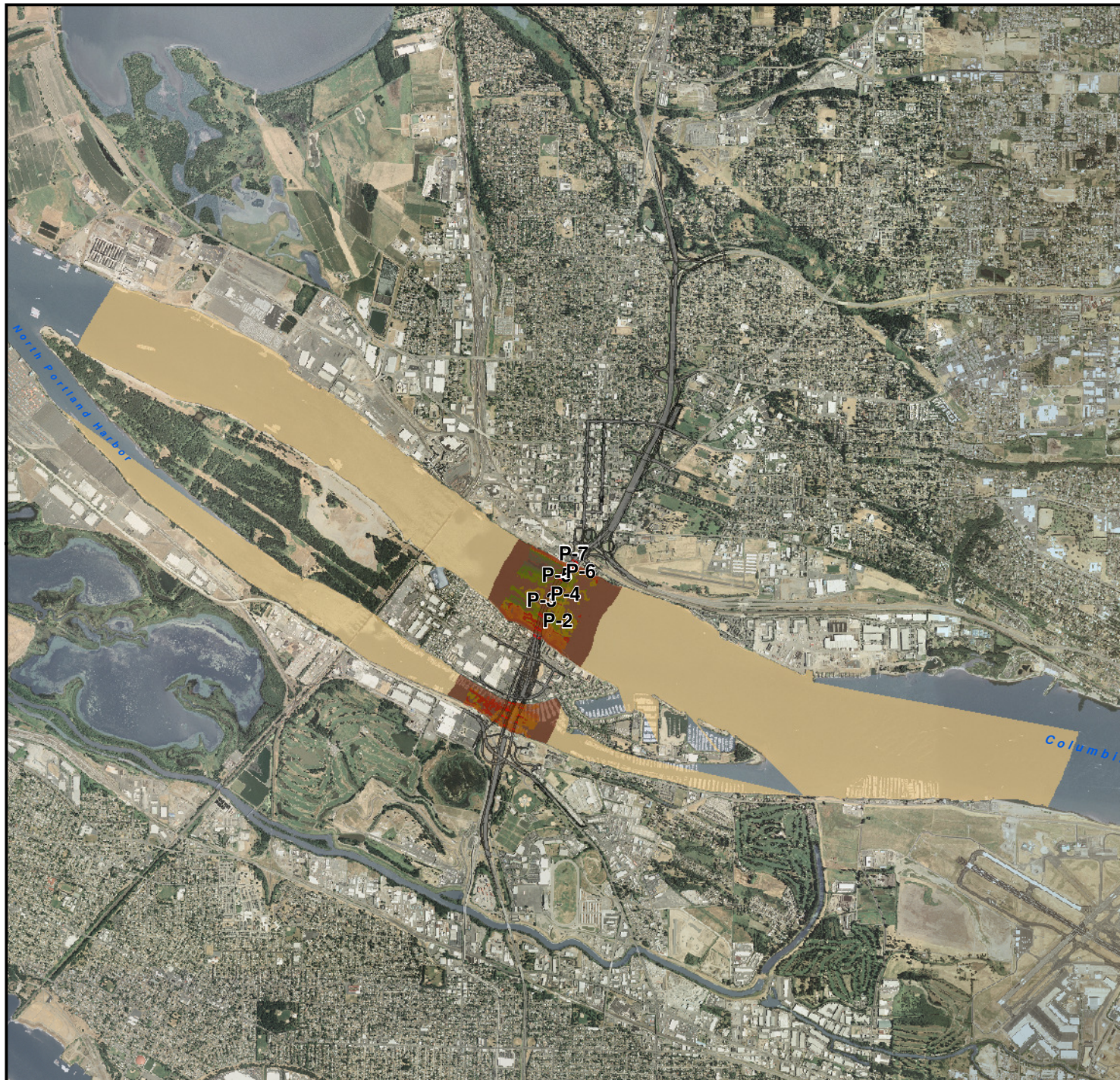
Exhibit 5-36. Extent of underwater impact pile-driving noise exceeding 160 dB RMS injury threshold for California and Steller sea lions, 36- to 48-inch pile.
