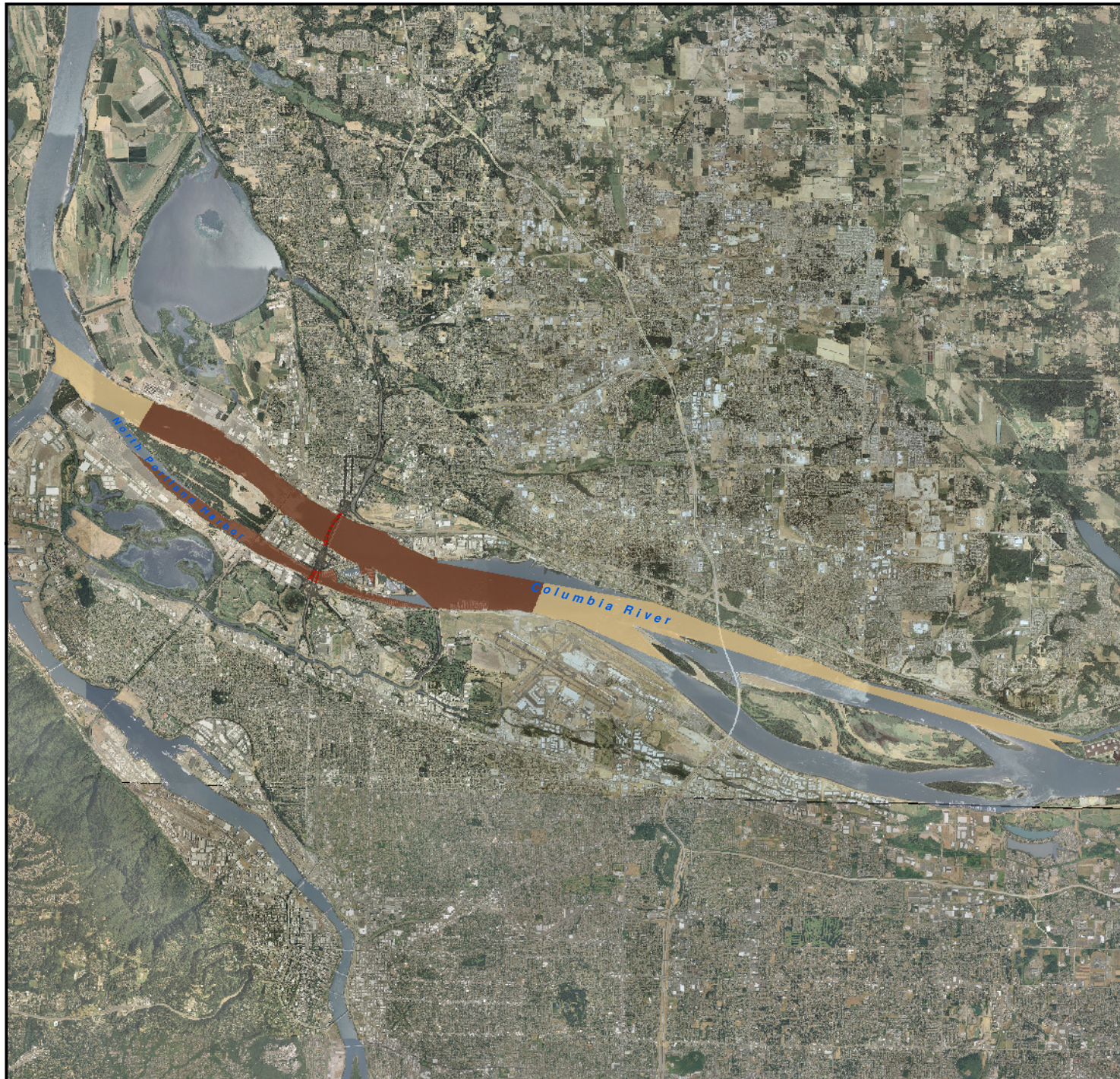
Exhibit 5-21. Extent of underwater impact pile-driving noise exceeding 150 dB RMS disturbance threshold for fish, 36- to 48-inch pile.
