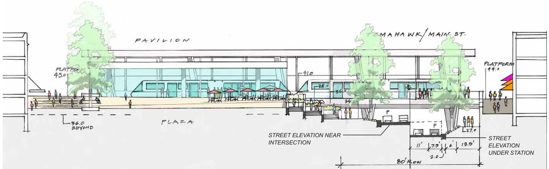
The Plaza Concept: Section looking east. (See red section line on page 25 for Tomahawk Island Drive elevations.) (Source: ZGF)
