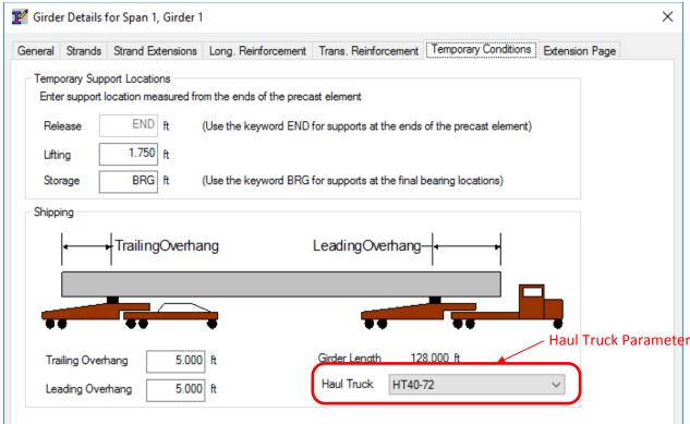
Figure 1 New Haul Truck Parameter
