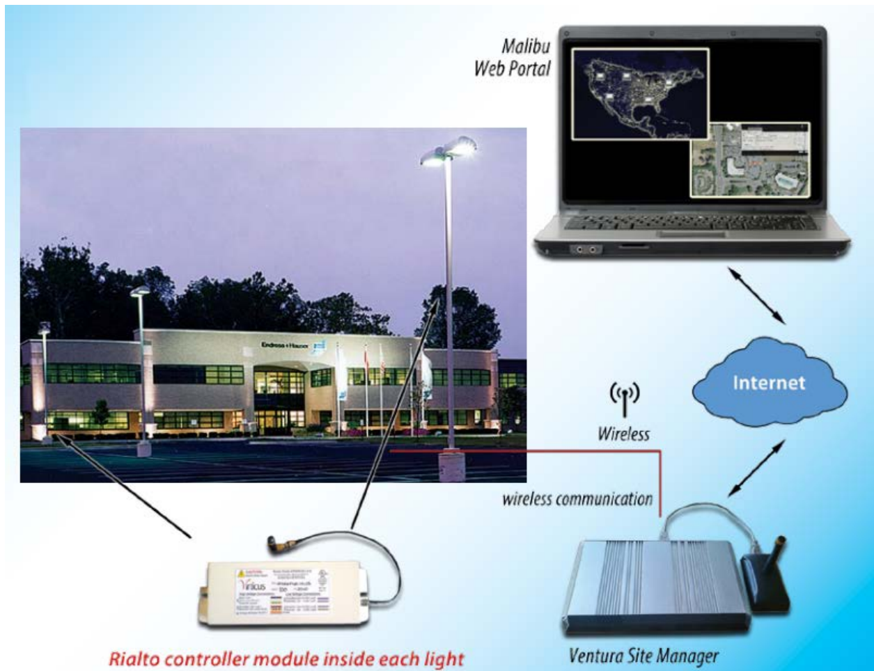
Figure 4-10 system architecture diagram for LSI Virticus (Source: LSI Virticus Network Architecture)
