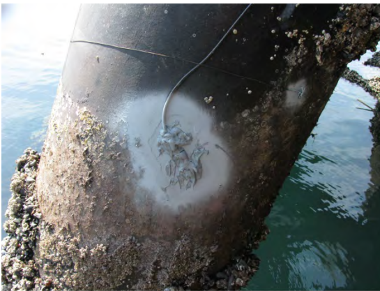
Figure 3.40: Installation of strain gauge (left) and distance sensor (right). Strain gauge covered in silicone and zinc-rich paint to protect against corrosive effects of saltwater. Distance sensor used to record vessel position measurements.
