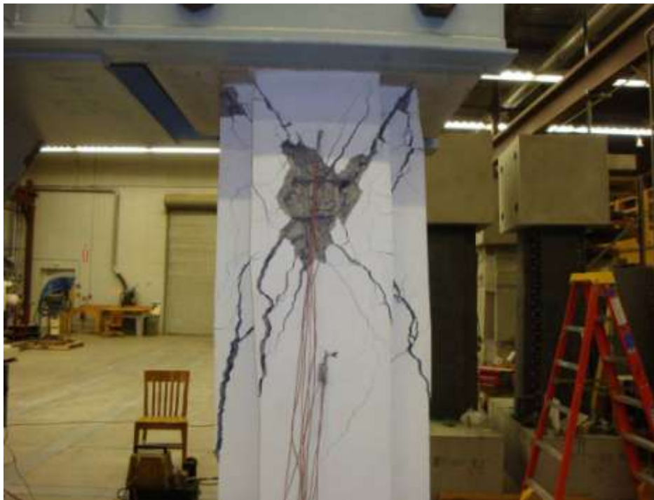
Figure 18 – Column 1 Shear Cracking Near the End of Testing
