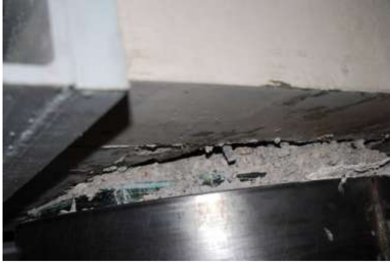
Figure 43 – Column 4 Longitudinal Rebar Fracture
