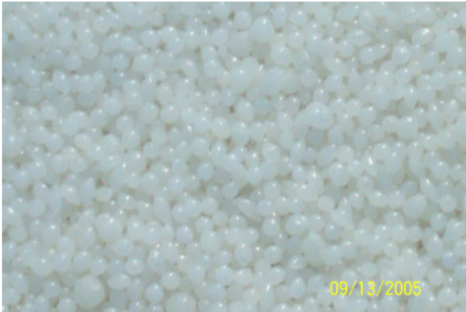
Figure 3.2: Sasobit wax pellets. [24]
