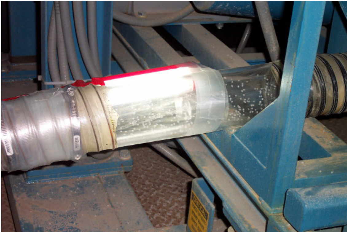
Figure 3.6: Sasobit flowing from distribution box to feeder tube. [24]
