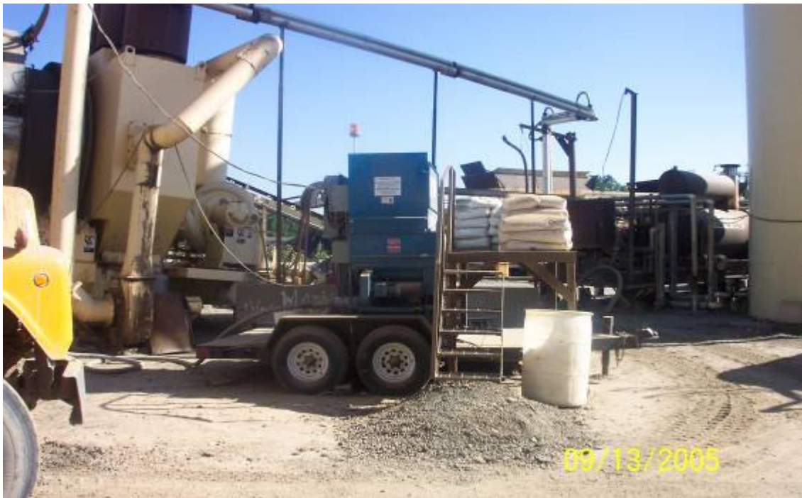
Figure 3.3: Pellet packets and distribution box (blue box in the center). [24]
