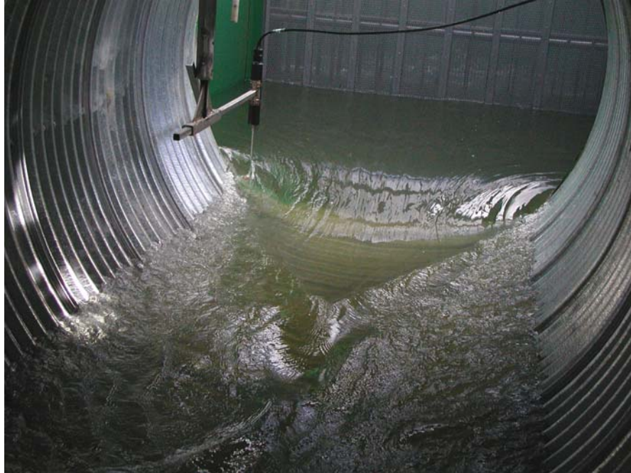
Figure 27. Picture of the Flow Conditions at the Culvert Inlet. Note that the reduced velocity zones at the culvert edges disappear near the culvert inlet at the HW tank.
