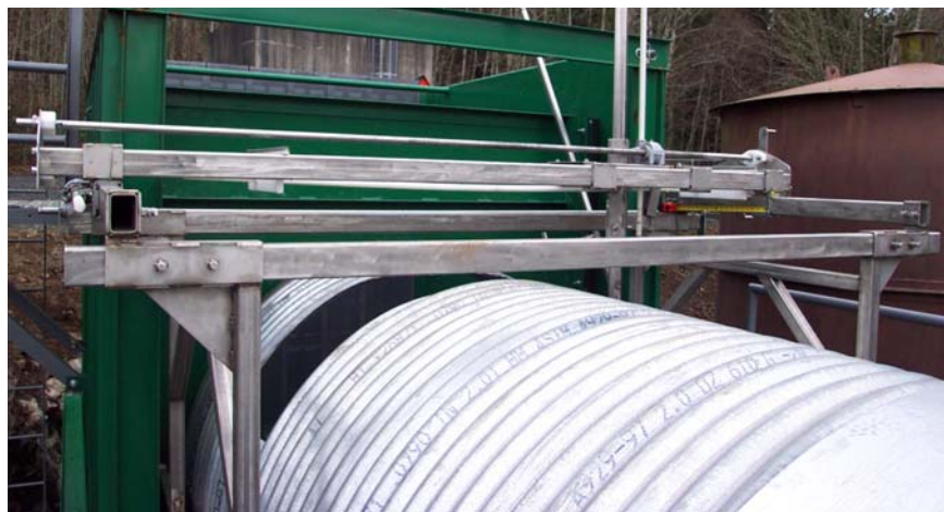
Figure 7. Three-axis Gantry Used to Position the ADV.
