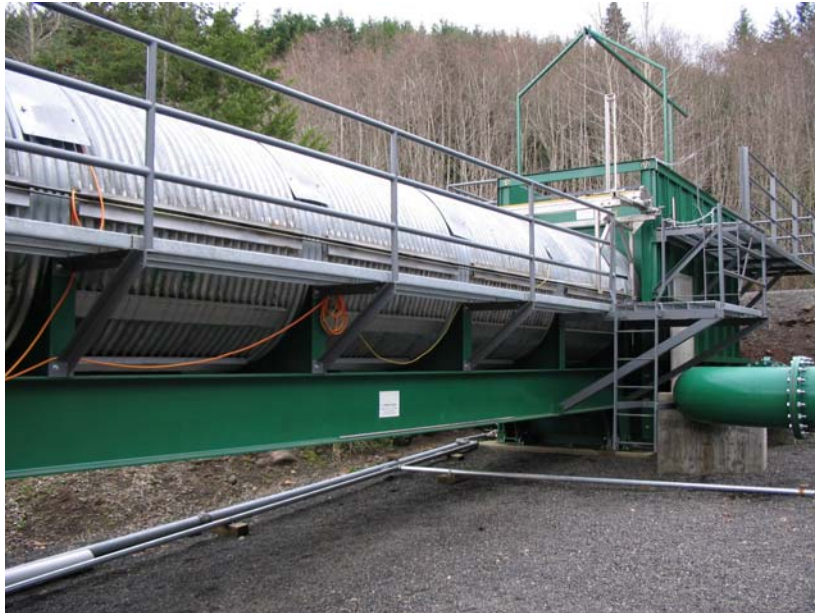
Figure 1. Culvert Test Bed. This photograph shows the culvert (foreground) and headwater tank (right side).
