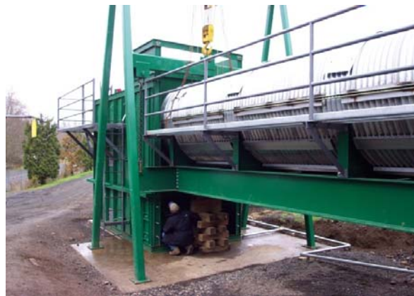
Figure 4. Culvert Test Bed Showing Tailwater Tank, A-frame, and Culvert Barrel.
