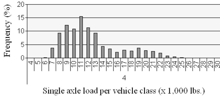
Figure D-1. Single axle load spectrum for Class 4 vehicles (Station P4N-2002)
