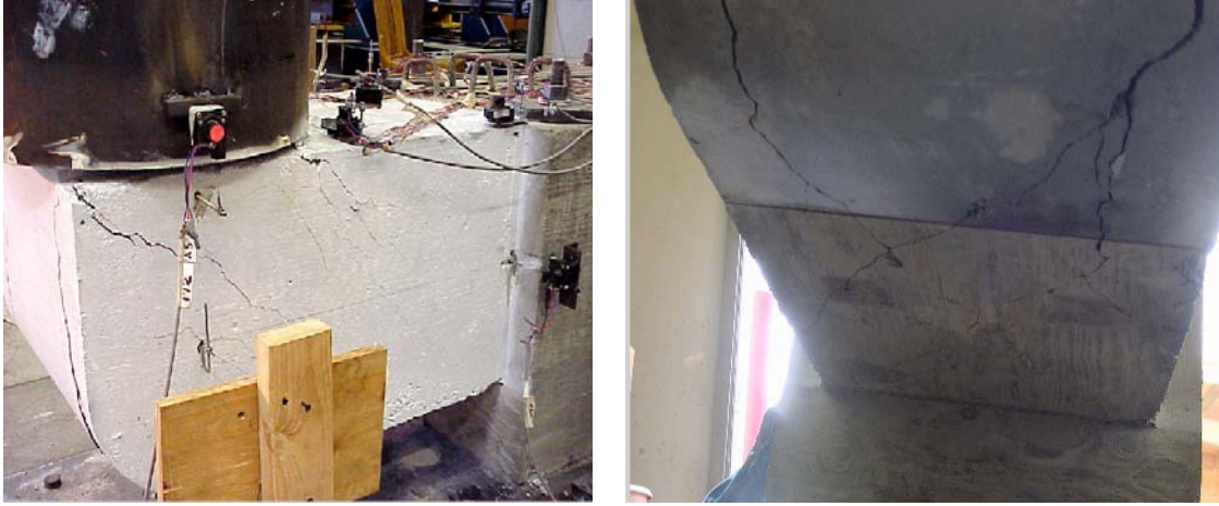
Figure 4-12: Torsion Cracks in “Short” Outrigger, Out-of-Plane Loading (Courtesy of Washington State University)
