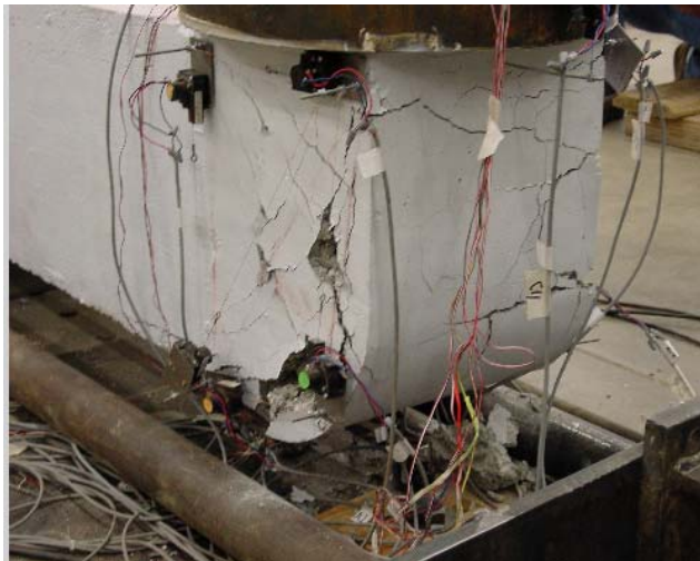
Figure 2-9: Damage to the “Long” Specimen Under In-Plane Loading ( Courtesy of Washington State University )
